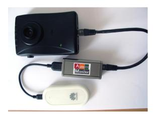
AutoMonitor Jump connected to Huawei E220 3G modem and IP camera
